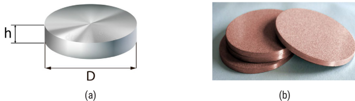
Figure 2. The schematic (a) and compacted Cu-Al-Ag (b) disc, where D=90.0 mm and h=10\pm0.5 mm.
